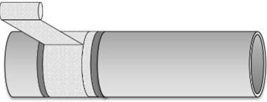
8) After the first new layer (layer three in total), if applicable, follow the directions in the following section to install the ILI Marker™ system at each end of the repair zone.
