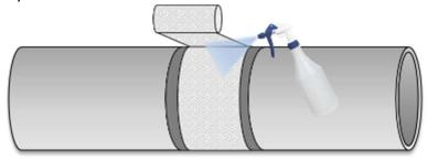
5) After the first layer, if applicable, follow the directions in the following section to install the ILI Marker™ system at each end of the repair zone.
