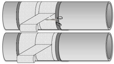
17) Continue this process until the entire repair zone has been wrapped. The last segment does not require a tie-in tab to be generated − rather, all layers should be lined up at the edge of the repair (allowing 2 inches of exposed adhesive primer to remain visible). Be sure to include ILI Markers™, if applicable, in the last segment on the first layer.
