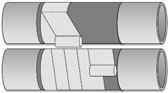
9) If the end of a roll is reached and more A+ Wrap<sup>™</sup> is required, open an additional roll and follow the same roll preparation procedure. Overlap the end of the previous roll by 4-6 inches with the new roll before continuing to wrap.
