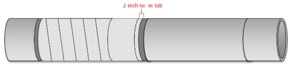
8) When starting the next segment, leave another 2 inch tie-in tab, if required. This segment will wrap over the initial tie-in tab.
