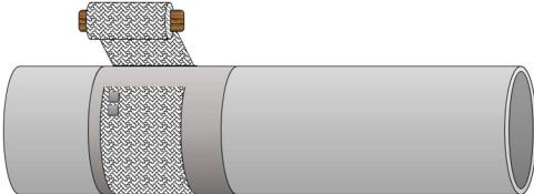
Note: It may be necessary to use a smaller width roll to ensure adequate space is available to install the Atlas<sup>™</sup> Carbon Fiber on. When applying fiberglass overlap the two layers with a minimum of one inch.
