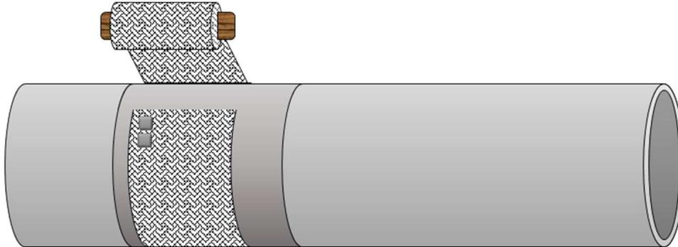
Note: It may be necessary to use a smaller width roll to ensure adequate space is available to install the Atlas™ Carbon Fiber on. When applying fiberglass overlap the two layers with a minimum of one inch.
