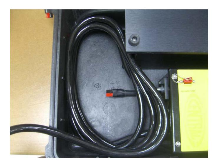
The key to this process is using all of the available space to wrap the cables.
