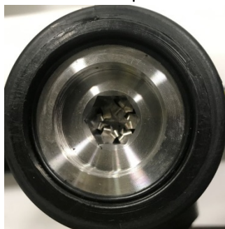
O-ring properly seated against punch
