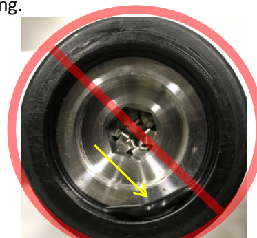
O-ring pinched and displaced
