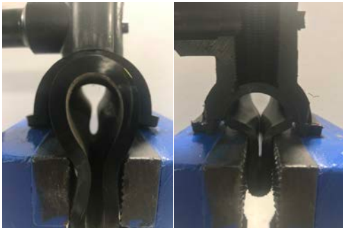
Saddle Crush Test – Passing Result
