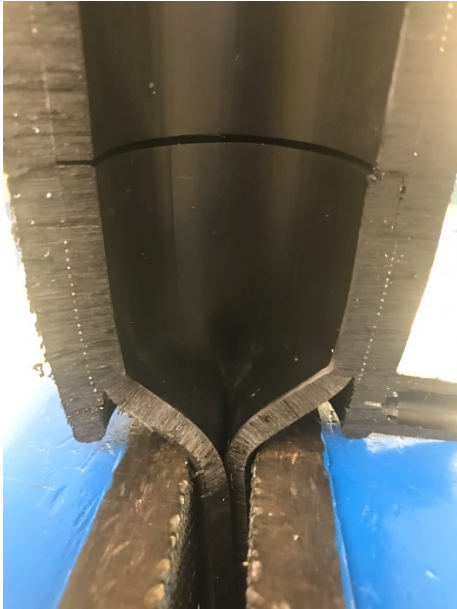
Coupling Crush Test - Passing Result
