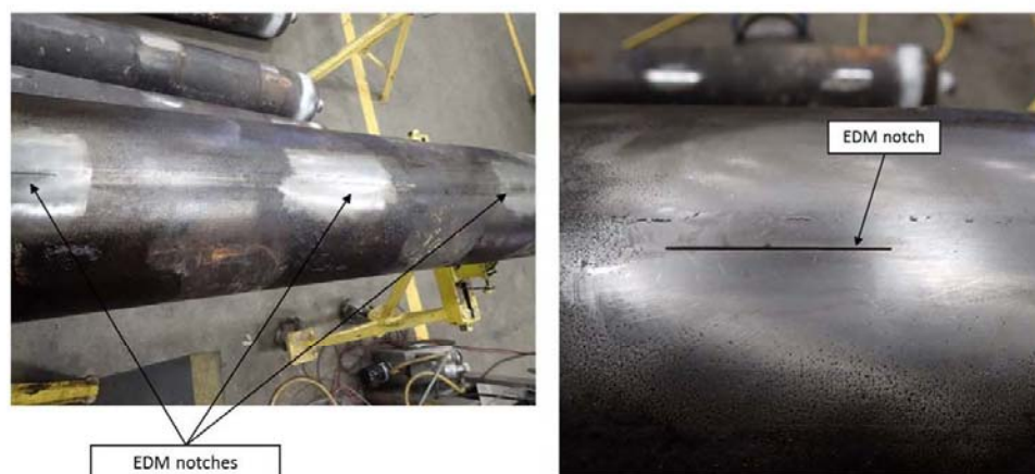
Figure 2: Photographs of EDM Notches
