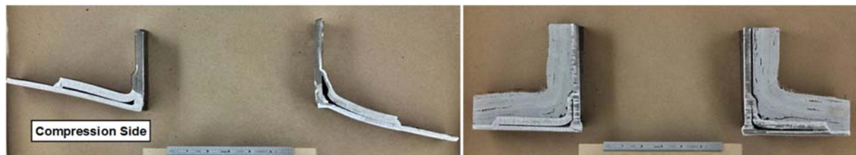
Unreinforced In-plane Sample (after 13.3 inches displacement at 88.6 kip-feet bending)
