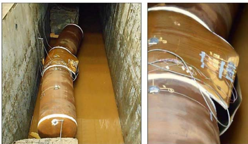
Figure 10: Burst test failure of unreinforced elbow sample
