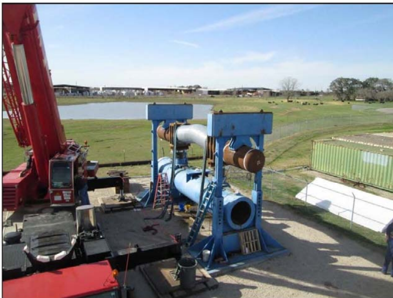
Figure 9: Aerial view of reinforced sample in bending load frame
