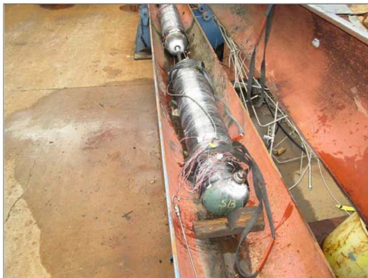
Figure 4: Milliken-Pipe Wrap Atlas System – as Repaired and Set up for Testing
