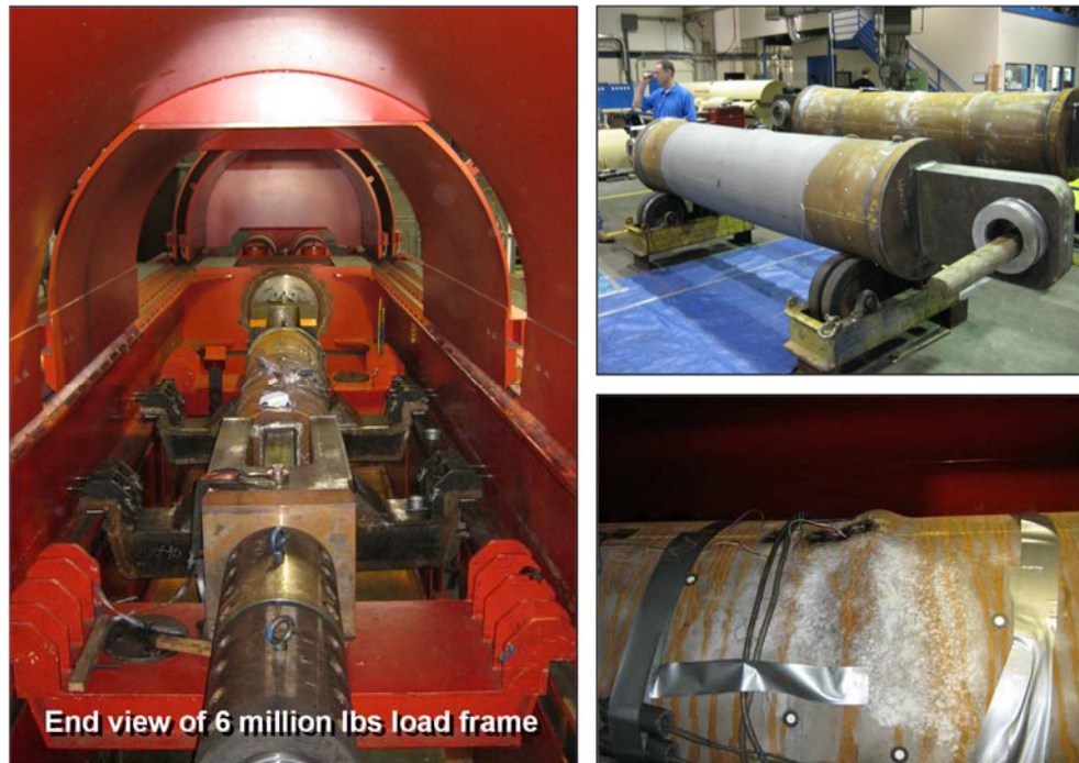
Figure 4-7: Photographs showing testing set-up for wrinkle bend testing
