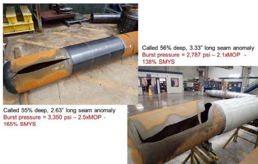
Figure 14: Photos Showing Burst Tests of Actual Reinforced Seam Planar Defects
