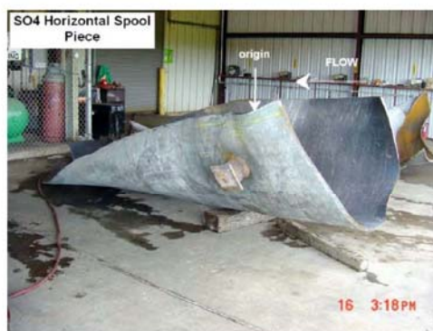
Figure 2: Horizontal spool piece showing fatigue-cracked seam weld
