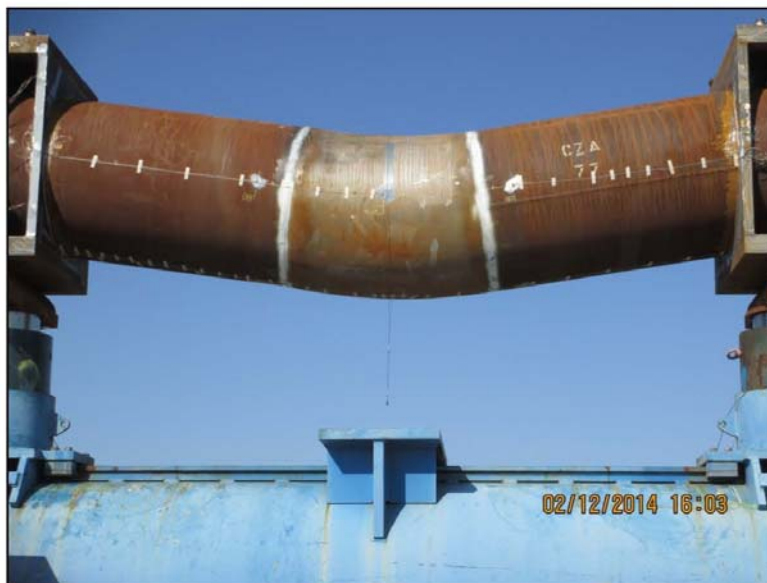
Figure 8: Close-up view of unreinforced sample on bending beam in OPEN mode
