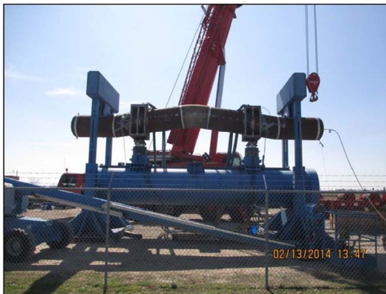
Figure 7: Unreinforced sample on bending beam in CLOSE mode
