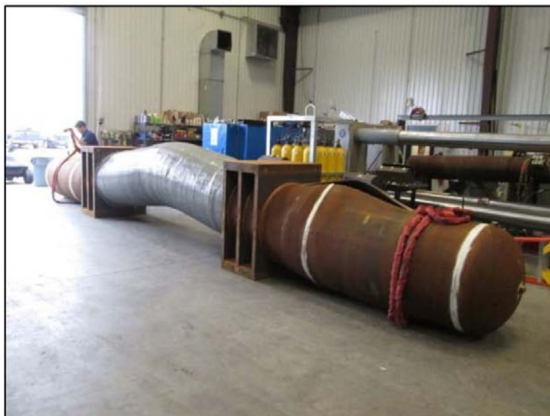
Figure 11: Burst test failure of reinforced elbow sample
