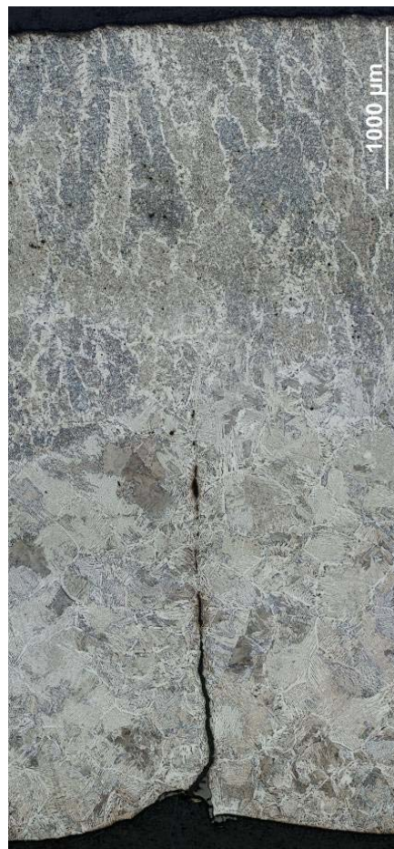
Figure 4-12: Metallographic section of the defective girth weld material
