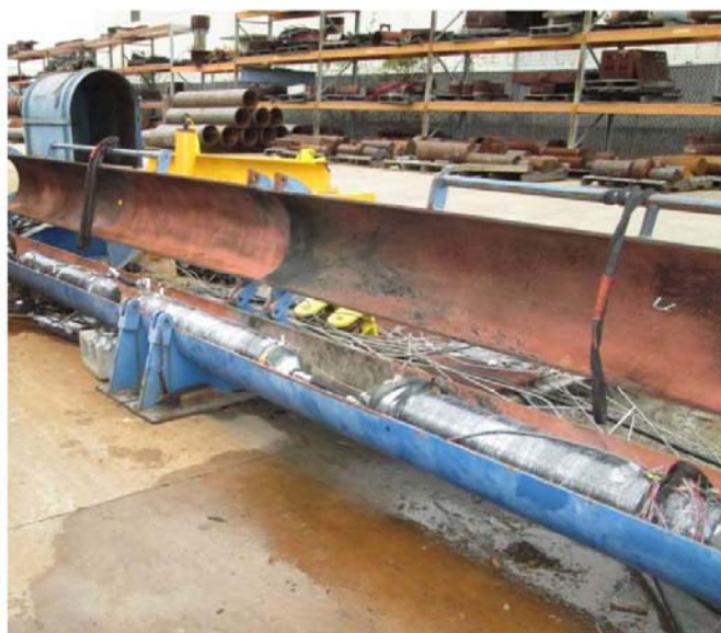
Figure 9: Photograph of Pipe Samples Installed for Pressure Cycling
