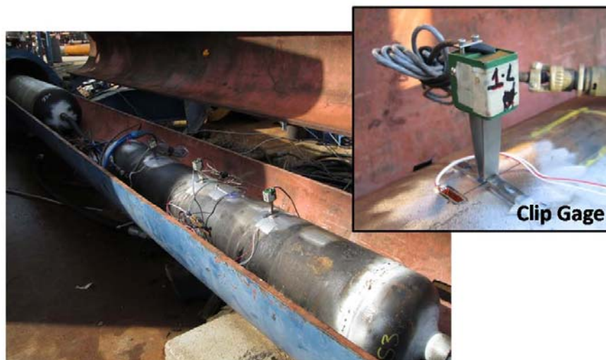
Figure 7: Photograph of Clip Gages on Unreinforced Samples
