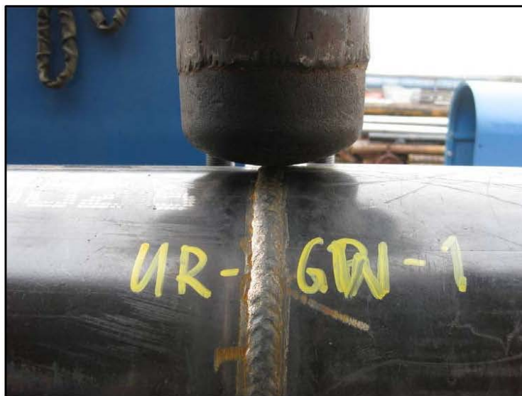
Figure 3 – Close-up view on indenter on girth weld
