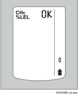
4. Close the test gas cylinder valve and remove the device from the calibration cradle.
