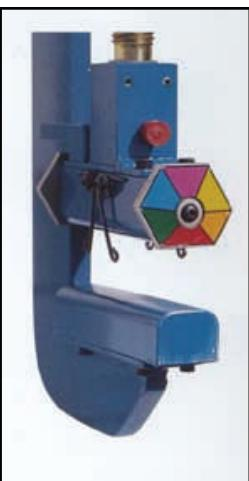
A unique feature of the GLS-26 is it's color-coded, stainless steel gap stop selector disc—This color coded disc is connected to a matching stainless steel gap stop disc by a 7/16" stainless steel hex shaft. As the color-coded gap stop selector disc is turned, it simultaneously turns the stainless steel gap stop disc located on the opposite side of the upper jaw. A spring and ball detent, provides positive gap stop placement with an audible click.
