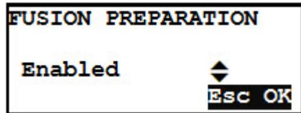
Select to enable or disable the assistance mode by using the (▲) (▼) keys and pushing START/OK (I) to confirm the setting. To cancel the operation press STOP/ESC (O).
