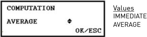
Immediate: What you get on the display is what the GPS sees at that time. In this case the data samples obtained are not manipulated, meaning that possible errors are not filtered out. These coordinates may not be as accurate as those calculated using the "Average" setting.
