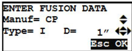
When all the proper data has been entered, press START/OK (I) to advance to the fusion process.
