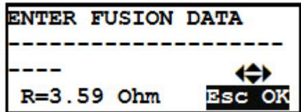
If the data cannot be read with the barcode wand for any reason, the user can manually enter the 24 digits printed on the barcode by pressing the (▶) button to go into “edit” mode and then using (▲) and (▼) to select the required digits. Once the 24 digits are entered, push START/OK (I).
