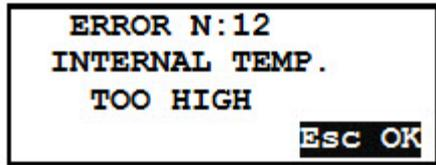
At this point, it will be necessary to allow the processor to cool down before a fusion can be attempted.
