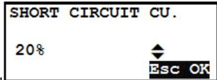
Select the desired short circuit value by using the (▲)(▼) buttons and pushing START/OK (I) to confirm the setting. To cancel the operation press STOP/ESC (O).
