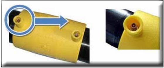
and the white connector end to the fitting post that is solid (no implanted resistor). Once the processor and fitting are properly connected, press the **START/OK (I)** button.
