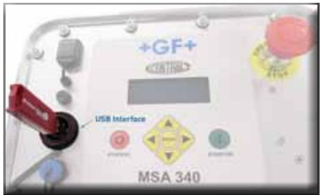
The connector is protected against dust and water by a cap, which ensures an IP65 protection factor when properly sealed.
