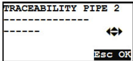
When all the traceability input data has been completed, the MSA displays a summary of the fusion parameters.
