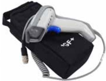
The barcode wand operates best when held at a perpendicular angle of 10–30 degrees and run across the barcode label in one continuous swipe (can be swiped forward or backwards on the label).
