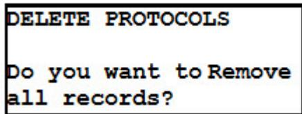
Press START/OK (I) to erase all fusion memory data. To cancel the operation press STOP/ESC (O).
