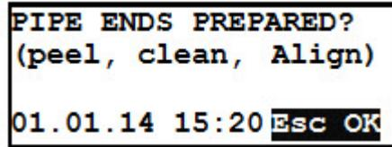
If the FUSION PREPARATION function is enabled, the display shows a message which asks for confirmation that all pipe preparations (scraping, cleaning, and alignment) has been done. If all pipe preparation is complete, press START/OK (I) to start the fusion process.
