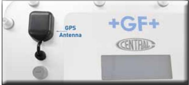
The acquisition of the coordinates is done just before starting the fusion process. At that time, the processor must be near the exact position where the fusion is to be performed.
