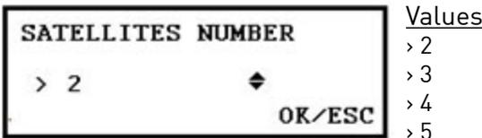
Keep in mind, that if this value is set to ">5", the GPS signal lock icon will not appear until the GPS receiver receives signal from 5 satellites. If the user is in an urban setting, with many tall obstructions or in a deep valley, getting 5 signals may be difficult.
