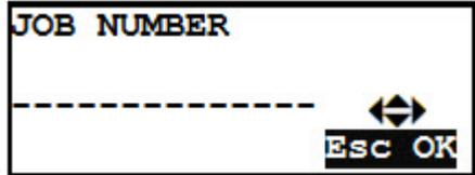
In the JOB NUMBER screen, the user can insert the current job code using the (▲) and (▼) buttons to select the desired character; the (◀) and (▶) buttons allow the movement of the cursor. To confirm, and move to the next page, push START/OK (I); to go back to the previous page push STOP/ESC (O).
