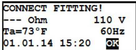
of the voltage value, '^^^' if the voltage is above the voltage limit threshold, or 'vvv' if the voltage is below the voltage limit threshold. In this case, the unit will stop the operation during the fusion if the input voltage does not return within the voltage threshold limit.
