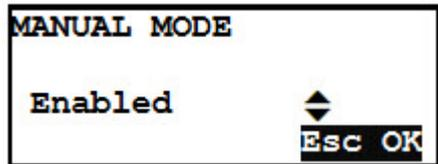
Select to enable or disable the assistance mode by using the (▲) (▼) buttons and pushing START/OK (I) to confirm the setting. To cancel the operation press STOP/ESC (O).
