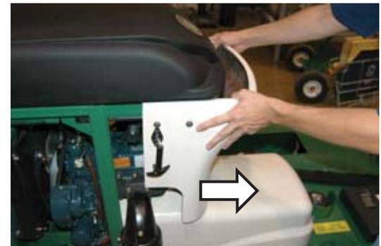
Loosen thumbscrew and remove the bottom cowl, sliding it forward then up.
