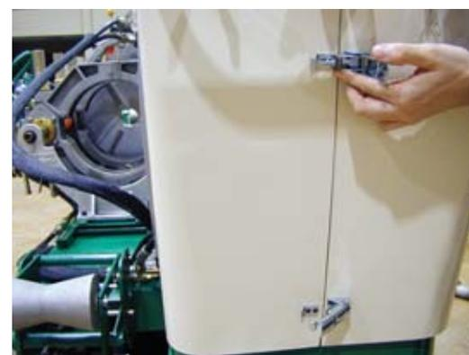
Align and fasten the front latch the same way.
