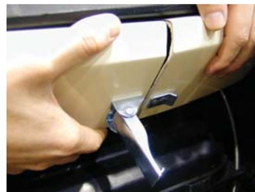
Reverse the procedure to remove the cowls.
