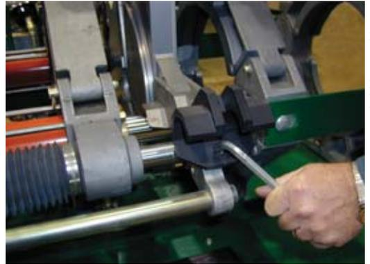
Support the facer with a person or sling so it does not fall once the facer locking bolts are removed.
