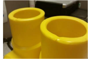
Figure 1 Example of dimple in the melt pattern
