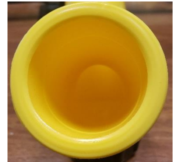
Figure 2 Example of melt surface unevenness
