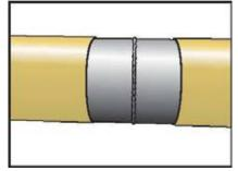
5. A 2.5-4 mil (63.5-101.6 micron) surface profile with sharp angularity. Burnishing or polishing must be avoided. Surface preparation can be controlled using surface profile tape. Dry surface and insure ideal surface preparation.
