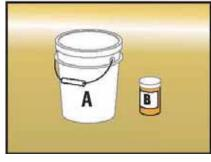
1. The 2-component epoxy coating is supplied in premeasured kits. Part A (large container) is the Base and Part B (small container) is the curing agent.
