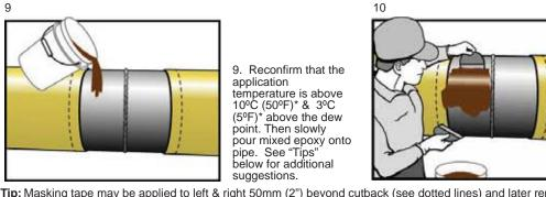
10. Use trowels. brush or roller to apply required minimum thickness of coating to the Field Joint. Cover at least 50mm (2") of the adjacent mainline coating.
