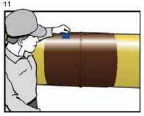
11. Use a Wet Film gauge to measure that the desired minimum thickness has been achieved. Double check around the weld to insure minimum desired thickness.
