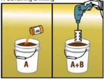
7. Warm parts A & B to 20°C (68°F) and mix by pouring all of part B into part A. Thoroughly scrape container and lid of B. Slowly begin mixing to avoid introducing air into the mixture.
