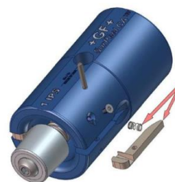
3. Remove Blade and Spring
