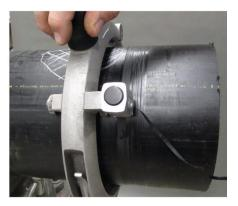
**Step 3:** Install correct fitting holder on the Top Load Clamp. If using a Tapping Tee, remove the cap from the fitting. For pipe sizes larger than 12", a 10" strap is included. Assure the straps are aligned with the outlet of the tee and the body. Straps wrapping around the pipe should not be twisted.
