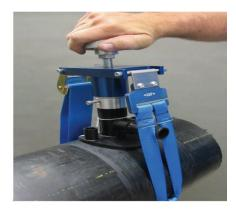
**Step 5:** Tighten until the indicator post (located in the center of the knob) is flush with the top of the knob.
