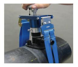
**Note:** Make sure that the knob is fully retracted before tightening the strap.
