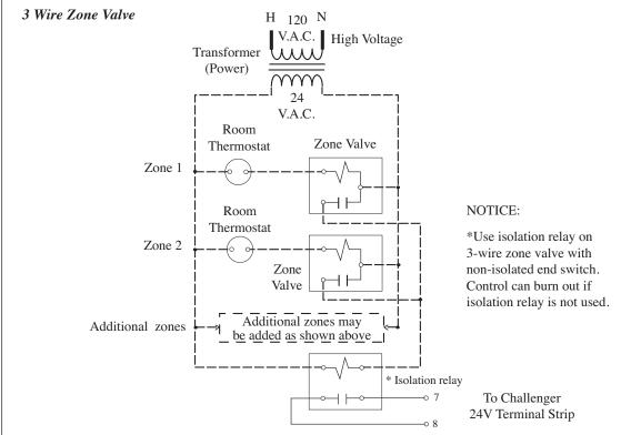
Fig. 19: Multiple Zone Field Wiring Using Zone Valves
