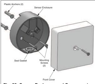
Fig. 22: Sensor Enclosure and Components
