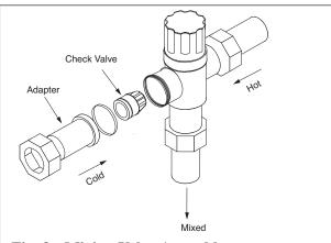
Fig. 9: Mixing Valve Assembly
