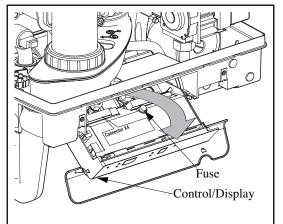
Fig. 17: Accessing Low Voltage X4 Connections
