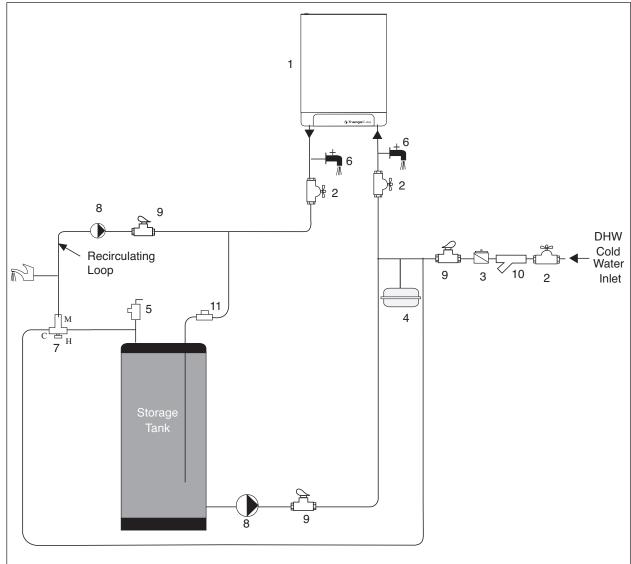
Fig. 12: Domestic Piping - Storage Tank Installations
