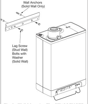
Fig. 2: Wall Mounting The CHALLENGER
