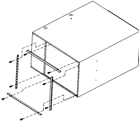
FOUR ANGLE BRACKETS ARE SHIPPED WITH EACH UNIT THAT CAN BE INSTALLED HORIZONTALLY. THESE BRACKETS MAY BE USED TO SECURE THE RETURN AIR DUCT TO A HORIZONTAL UNIT.
