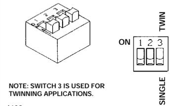
NOTE: SWITCH 3 IS USED FOR TWINNING APPLICATIONS.
