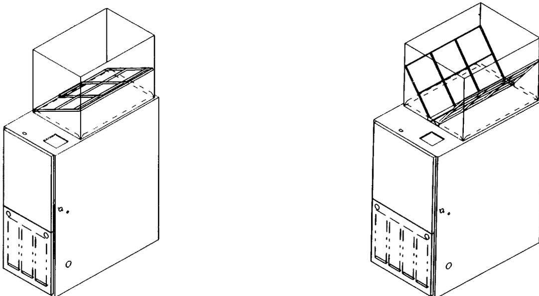
**IMPORTANT:** Do not operate the system for extended periods without filters. A portion of the dust entrained in the air may temporarily lodge in the air duct runs and at the supply registers. Any recirculated dust particles will be heated and charred by contact with the furnace heat exchanger. This residue will soil ceilings, walls, drapes, carpets, and other household articles.
