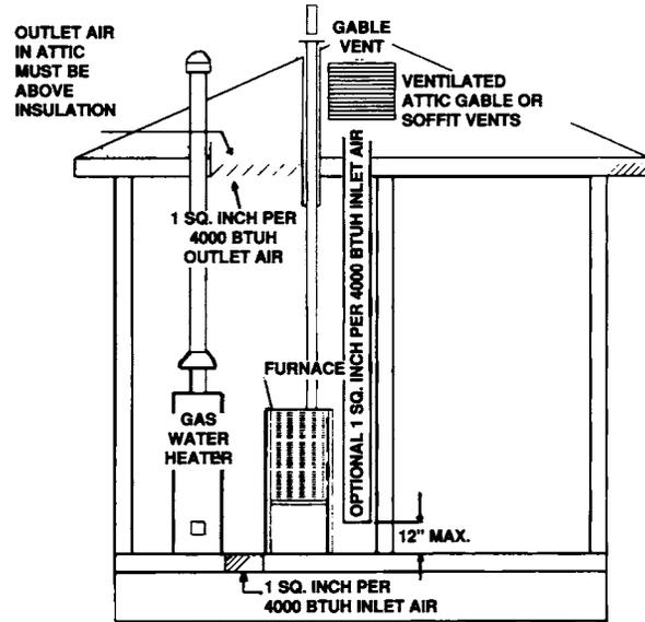
**EXAMPLE 2. FURNACE LOCATED IN A CONFINED SPACE**
