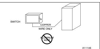
Use a separate, fused branch electrical circuit with a properly sized fuse or circuit breaker for this furnace. See **Table 11** for wire size and fuse specifications. A readily accessible means of electrical disconnect must be located within sight of the furnace.
