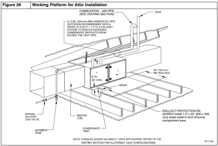
NOTE: Local codes may require a drain pan and condensate trap when a condensing furnace is installed over a finished ceiling
