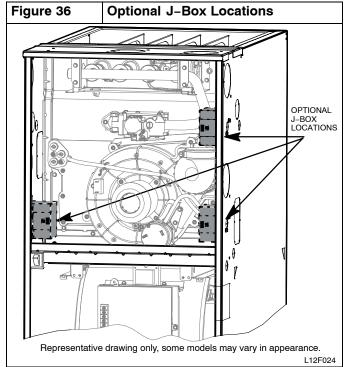
Remove the J-Box cover and mounting bracket from the loose parts bag. Select a 7/8-in. (22 mm) knock-out on the desired side of the casing. Remove the knock-out from the casing. Drill two 1/8-in. (3 mm) pilot holes in the casing dimples by the desired 7/8-in. (22 mm) knock-out.
