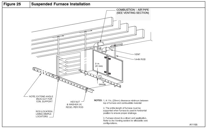
NOTE: Local codes may require a drain pan and condensate trap when a condensing furnace is installed over a finished ceiling
