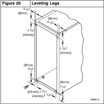
**NOTE**: Bottom closure must be used when leveling legs are used. It may be necessary to remove and reinstall bottom closure panel to install leveling legs. To remove bottom closure panel, see Step 1 in Bottom Return Air Inlet section.
