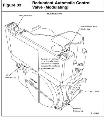
If pressure exceeds 0.5 psig (14-in. w.c.), gas supply pipe must be disconnected from furnace and capped before and during supply pipe pressure test. If test pressure is equal to or less than 0.5 psig (14-in. w.c.), turn off electric shutoff switch located on furnace gas control valve and accessible manual equipment shutoff valve before and during supply pipe pressure test. After all connections have been made, purge lines and check for leakage at furnace prior to operating furnace.
